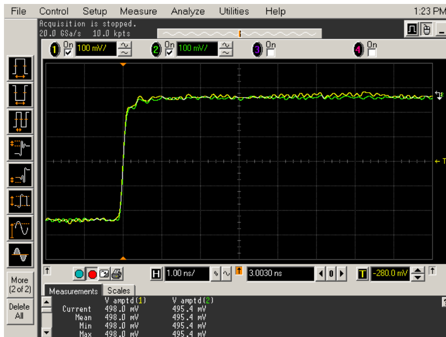
Figure 59 Calibration Probe Waveform Example
