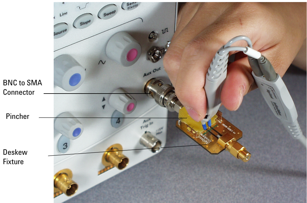
Figure 60 Browser Probe Head Calibration Connection Example
